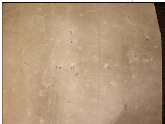
Figure 5 - Witness marks on Surface of Topcoat
