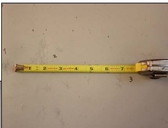
Figure 6 (Left) - Damage on back of membrane sample
